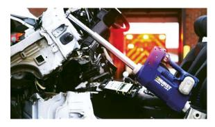
Rescue Ram pushed a dashboard forward in an automobile. Rescue Ram lifts dash for easy access to driver.
